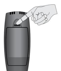
Open the back of the remote control. Push the retaining clip toward the cover then pull away from the remote control.
